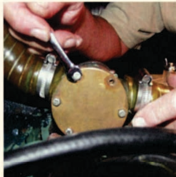
1 The original water pump cover is held in place with six set screws
