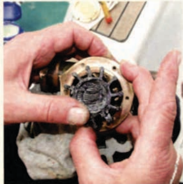
3 Impeller vanes must face the right direction when pushed inside the water pump body
