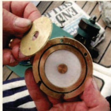
2 The replacement Speedseal cover features a PTFE washer and rubber O-ring seal
