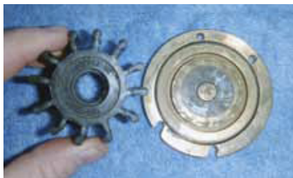
The Speedseal Life kit installed on our test boat's engine looked as good as new when we removed it after 73 engine hours.
