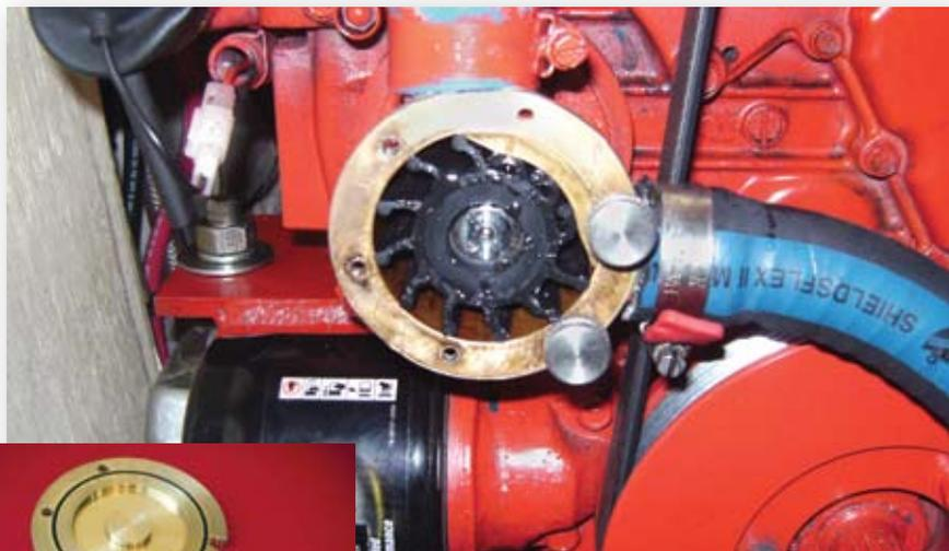
*PS installed the SpeedsealLife on our Union 36's water pump (above). Kits (left) include four hand screws, a brass cover and washer, and a Teflon washer.*
